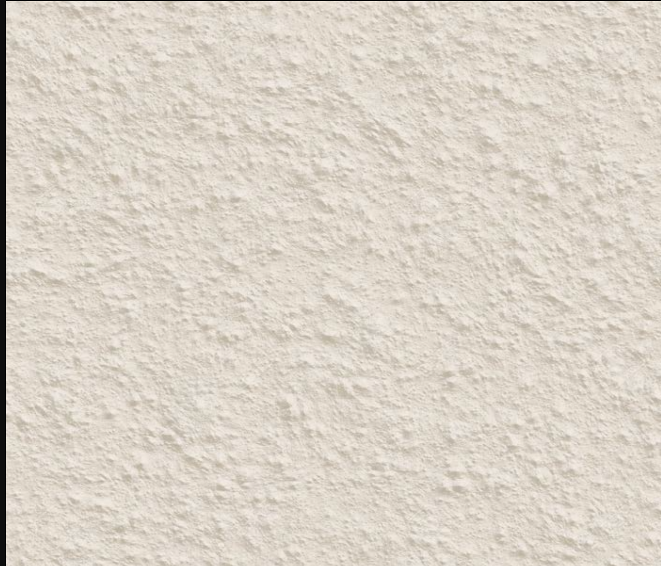
STUCCO SYSTEM MANUFACTURER: DRYVIT PROFILE: CCP-2 SYTEM, SANDPEBBLE FINE E FINISH COLOR: PAINTED, ALLURING WHITE SW6343
